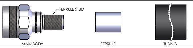
Cut end of cable evenly. Strip cable to dimensions shown. All cuts are to be clean and square. Do not nick braid, dielectric or center conductor. Add a chamfer to cable center conductor using a fine file or a sharpening tool.
