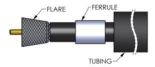
Slide ferrule stud under the braid until it stops. Slide ferule over braid.
